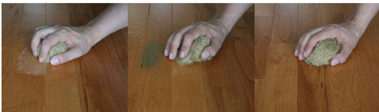
Fig. 7: Surface scratches on a UV surface with normal UV top coat
