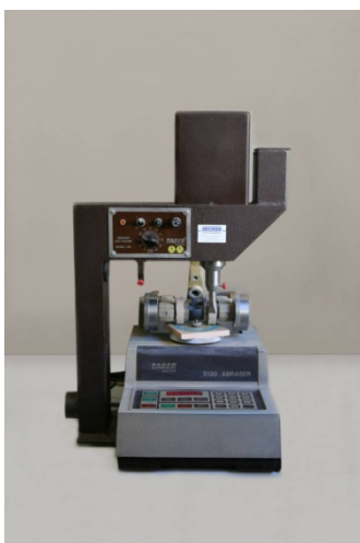
Fig. 17: Taber Abraser with falling sand device
