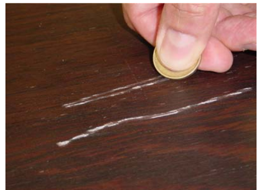
Fig. 2: Surface with bad adhesion after coin-test
