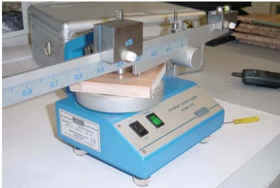
Fig. 10: Test device for measuring resistance to indentation
