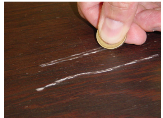
Fig. 2: Surface with bad adhesion after coin-test
