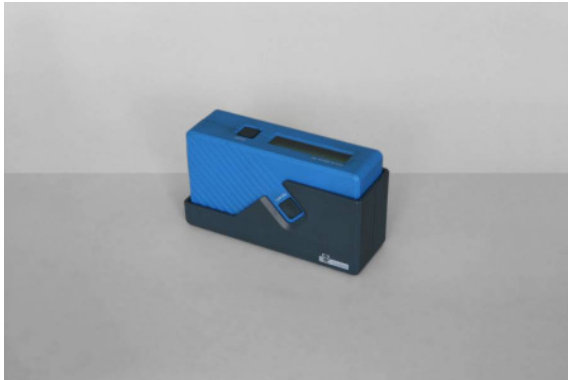
Fig. 6: Gloss value test device
