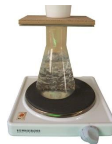
Fig. 21: Hot vapor steam test
