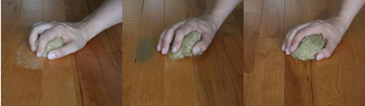
Fig. 7: Surface scratches on a UV surface with normal UV top coat
