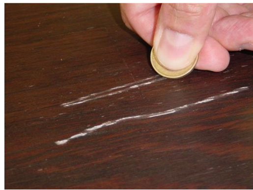
Fig. 2: Surface with bad adhesion after coin-test
